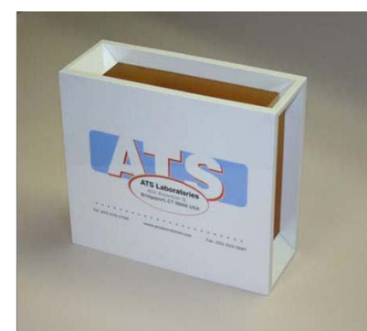
Fig. 1 Outward appearance and target diagram of the standardized phantom. It has 4 scanning surfaces and many internal structures with which various measurement can be performed.
